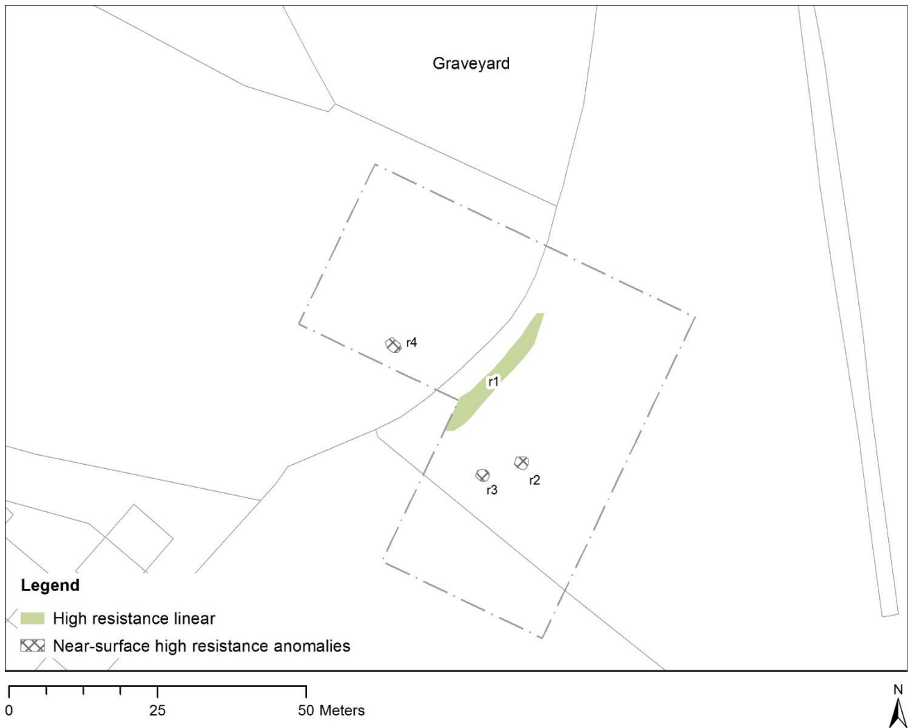
Figure 3 Interpretation diagram with geophysical anomalies identified
