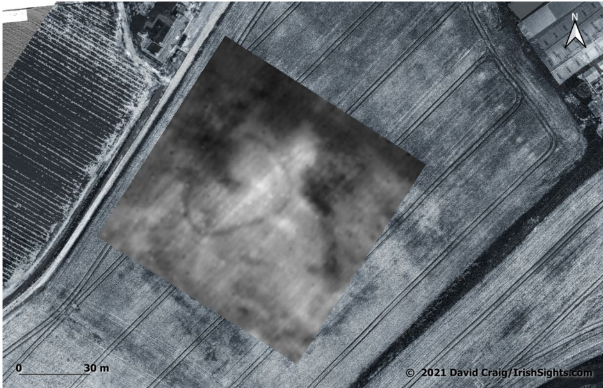
Figure 10: Resistivity plot overlay on adjusted drone orthomosaic
