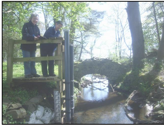
Figure 03: Members of survey team inspect a depth gauge down-stream of the stone bridge.
